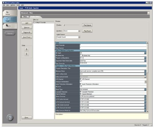
The Input Channels field tells the Dolby-e filter the number of audio channels available in the source file. The Start Channel field informs the filter where to begin the mapping of the 8-channels to the target.
